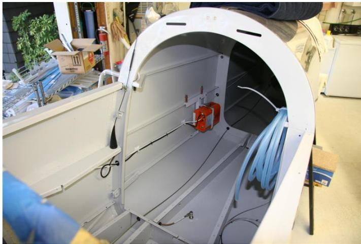
An ELT (the orange box) installed in a light plane.
