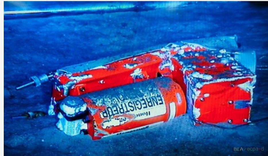
Cockpit Voice Recorder (CVR) capsule with the ULB still attached, but antenna broken off.
