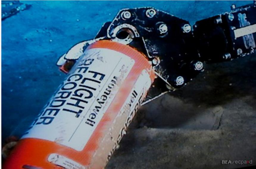
Flight Data Recorder (FDR) being recovered by a mechanical arm on the Remora 6000 Remotely Operated Vehicle; it was found *without* the Underwater Locator Beacon (ULB) chassis.
